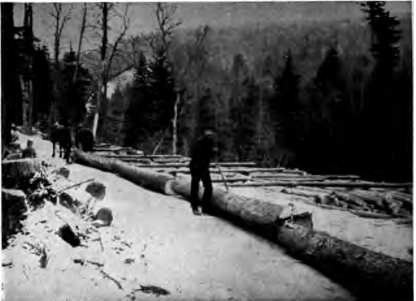
FIG. 31. — A Turn of Logs at the Dump along a Skipper Road. The logs are fastened together with "single coupler" grabs. West Virginia.
